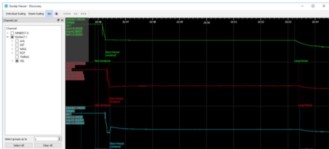
When the auto-centring is enabled, the centring procedure is activated as soon as the percentage reaches  $\pm 100\%$ . To turn off Automatic Mass Centring, select the  button in the Auto Centring option (not recommended). To restore the default setting, click on the  button.
