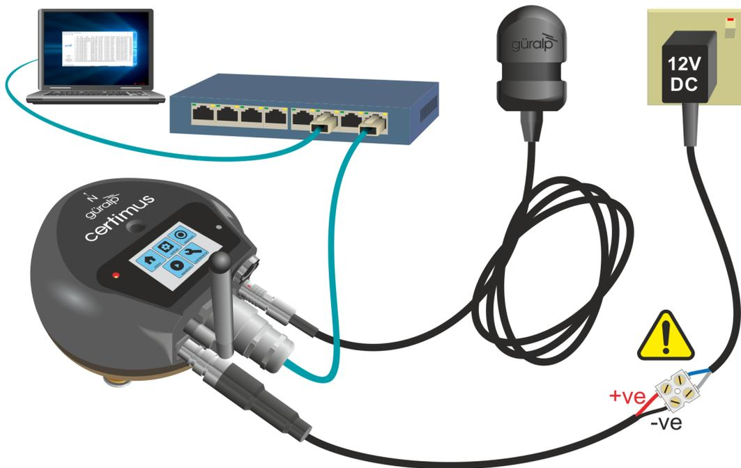
To get started, connect the cables as shown in the figure above and as described in Section 3.2 on page 18.
