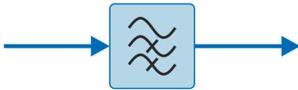
The output is the difference between a low-pass filtered copy of the signal and the unfiltered signal.
