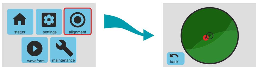
The red circle behaves like the bubble in a traditional bubble-level, moving towards the highest edge of the instrument. The further from the centre it is, the more adjustment is needed.
