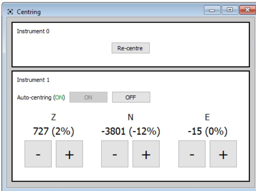
The mass position values in counts of the three components are showed in real-time under the corresponding component indicators (Z, N, E).
