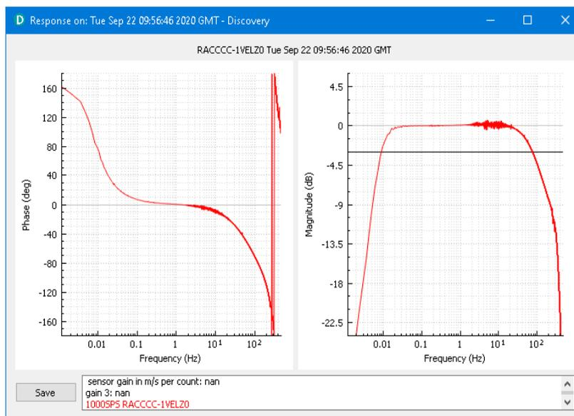
Calibration is a procedure used to verify or measure the frequency response and sensitivity of a sensor. It establishes the relationship between actual ground motion and the corresponding output voltage. Calibration values, or response parameters, are the results of such procedures.
