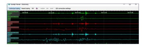
Signal statistics, measurements and comparisons can be performed with ease.
