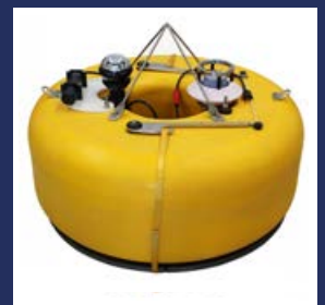
AQUARIUS AND MARIS ARE BOTH FULLY OPERATIONAL AT ±90 ° TO FACILITATE EASIER DEPLOYMENT ON THE SEAFLOOR
