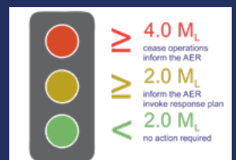
EXAMPLE MONITORING THRESHOLDS FOR TRAFFIC LIGHT SYSTEMS
